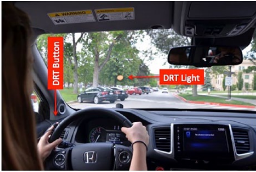
Figure 1. A research participant driving the 2017 Honda Ridgeline. Note the orange DRT light projected onto the windshield in the driver's forward field of view and the DRT microswitch attached to the participant's left index finger. The vibrotactile device attached to the participant's collarbone is not shown in the photo. DRT = Detection Response Task.
